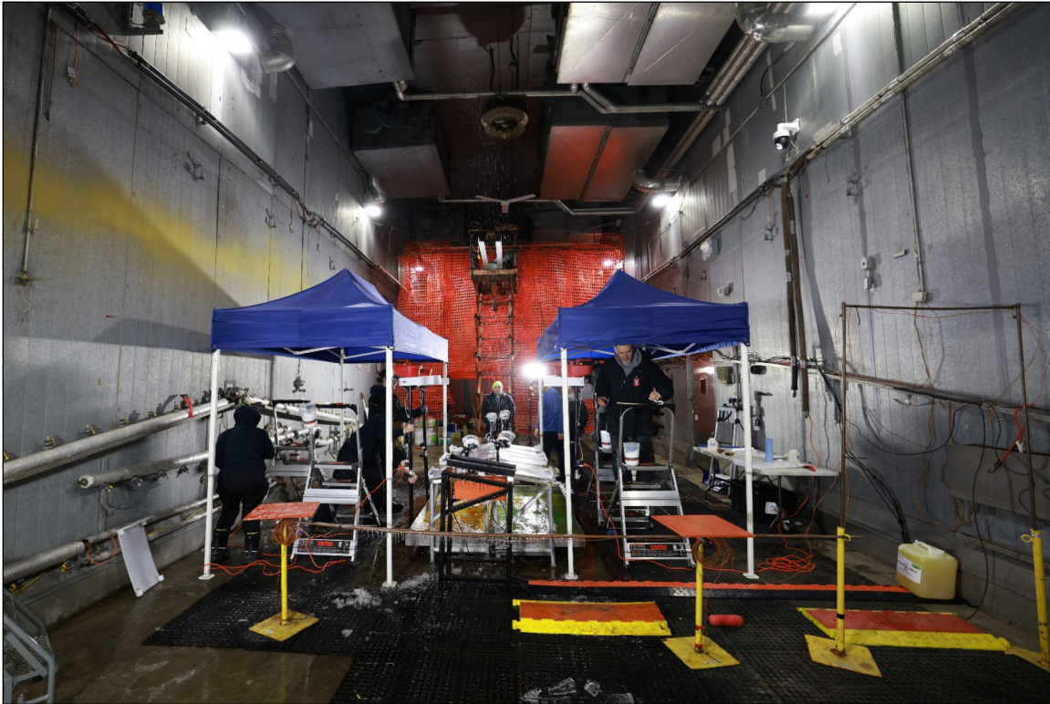
Photo 2.3: NRC CEF Cold Chamber and General Mixed Condition Testing Setup
