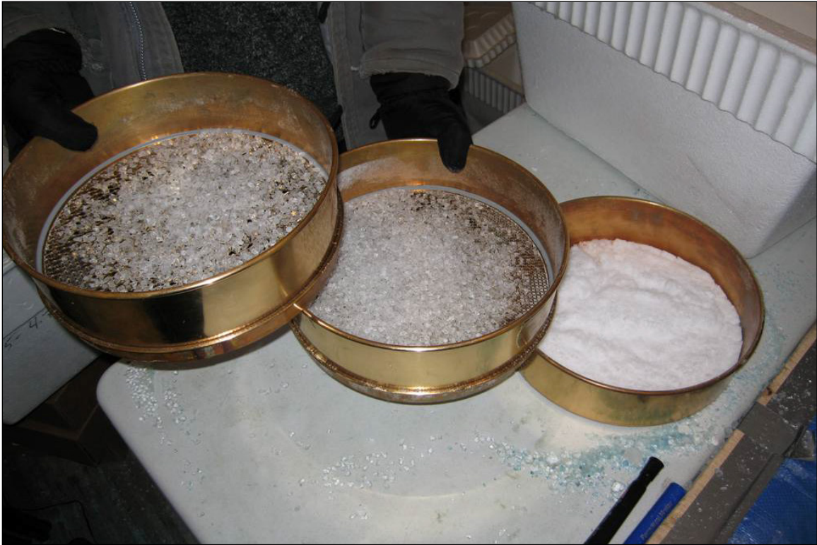
Photo 2.5: Calibrated Sieves Used to Obtain Desired Snow Size Distribution
