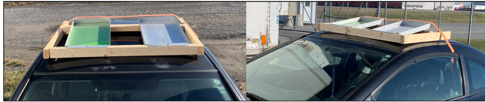
Photo 5.1: Example of Rate Pans Installed on a Test Vehicle
