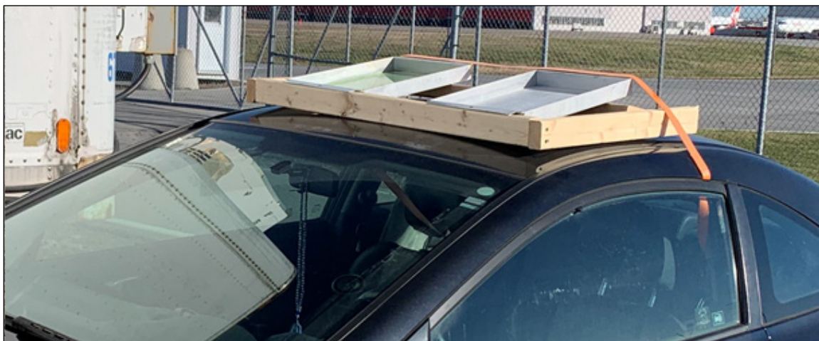
Photo 3.6: Method 1 – Simulated Taxiing Aircraft – Addition of Dry Pan Next to Wet Pan
