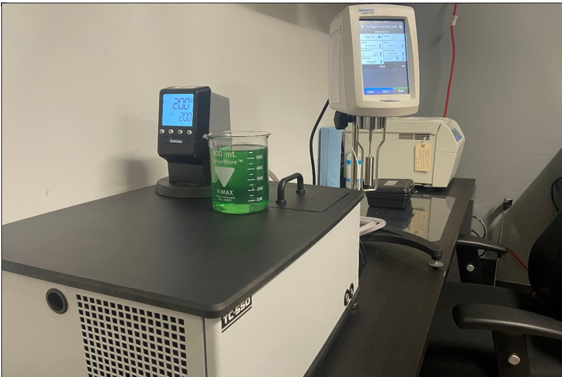
Photo 2.12: Brookfield® Digital Viscometer and Recirculating Bath
