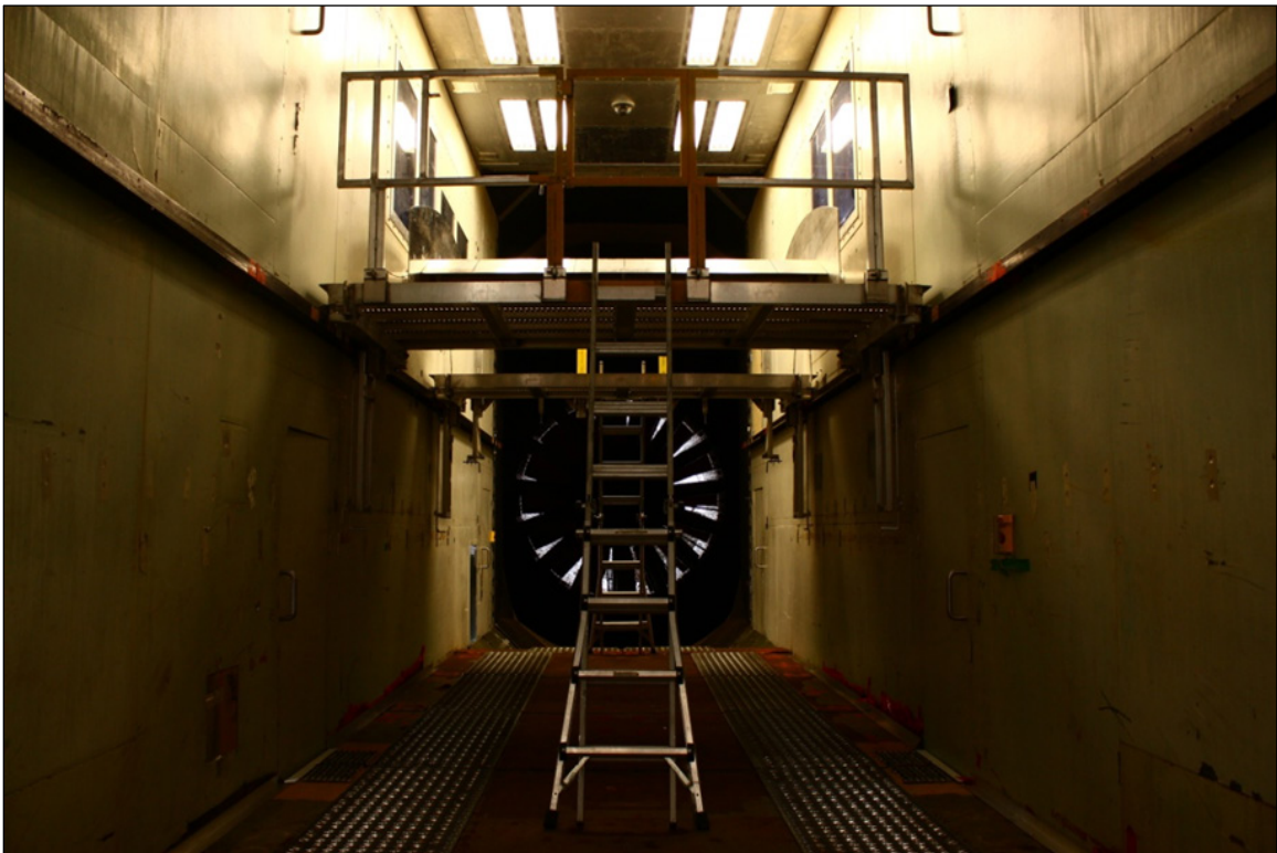
Photo 2.2: Inside View of the NRC Wind Tunnel Test Section
