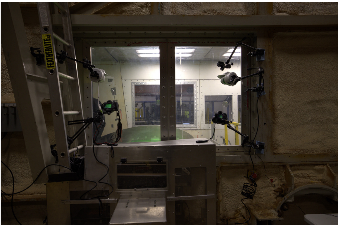
Photo 2.10: Wind Tunnel Setup for Digital Cameras
