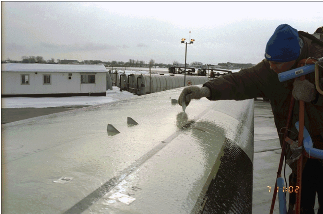
Photo 4.10: Appearance of Fluid Layer Prior to Propeller Run
