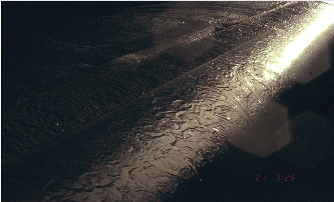
t = 3:26 AM, entire wing failed
