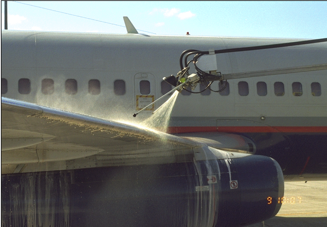
Photo 3.7: Elephant \beta – Standard Nozzle – Adjusted to Reduced Pattern
