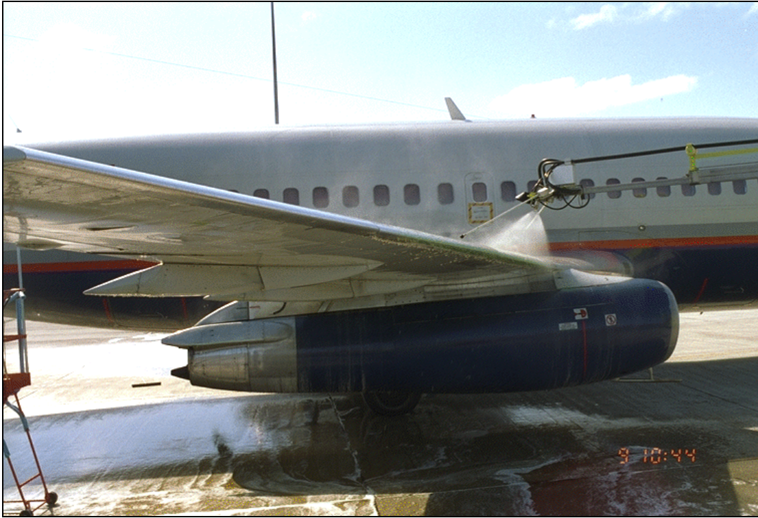
Photo 3.13: Elephant \beta – Optional Fixed Nozzle – Ultimate Thickness Trial
