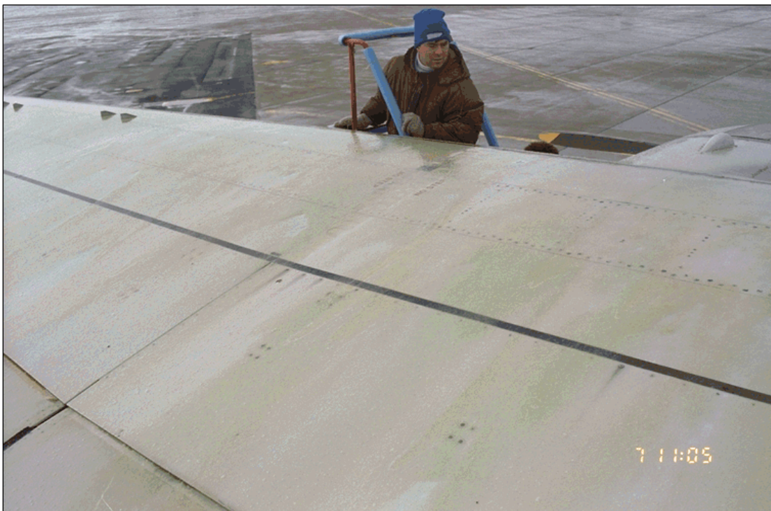
Photo 4.11: Appearance of Fluid Following Propeller Run
