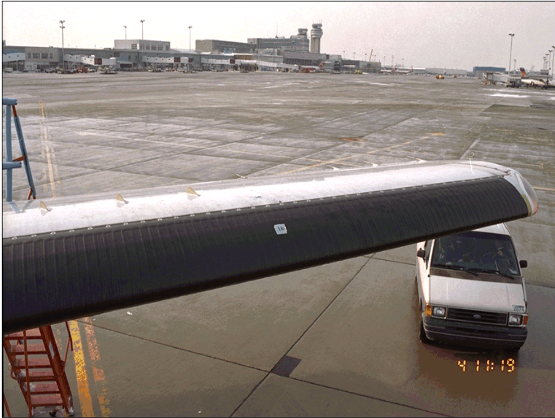
Photo 2.27: ATR 42 Wing – Ribbed Deicing Boot
