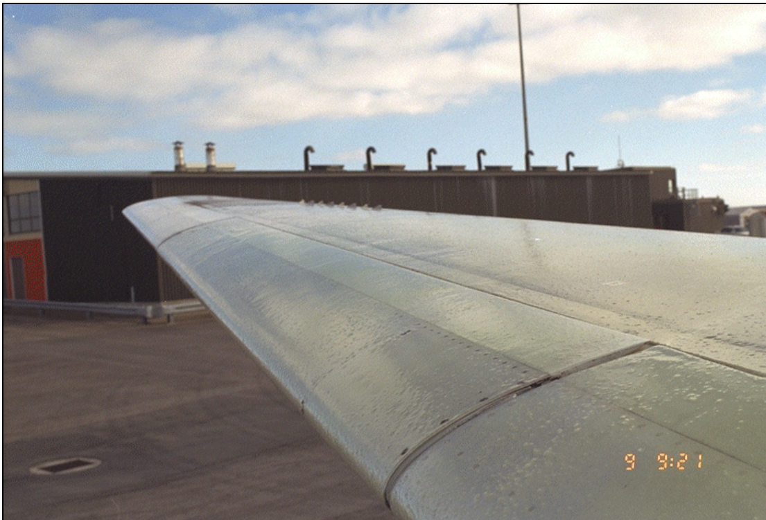
Photo 3.2: Nepiro Nozzle – Type IV Fluid After 20 Minutes
