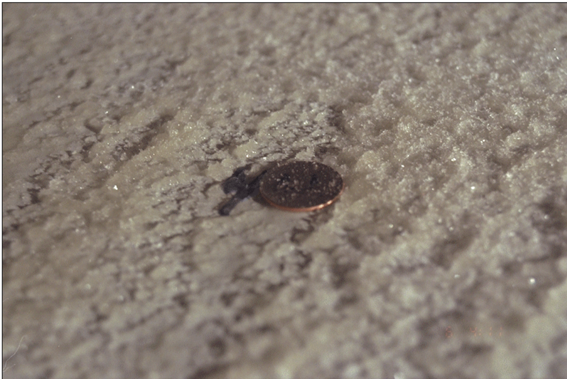
ID # 34, March 6, 1997, Fokker 100, t = 4:11 AM, 10% wing failure time was 4:10 AM, mid-wing, location 4
