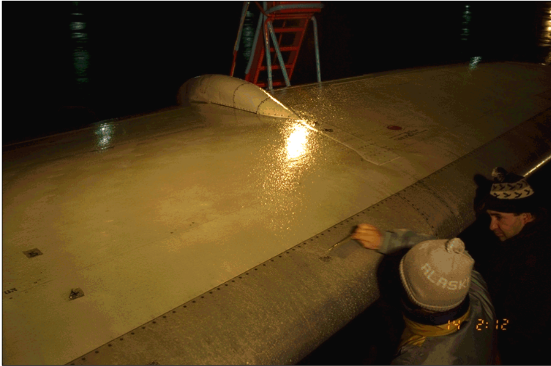
Photo 2.13: Fluid Sampling Location on Fokker 100 Wing
