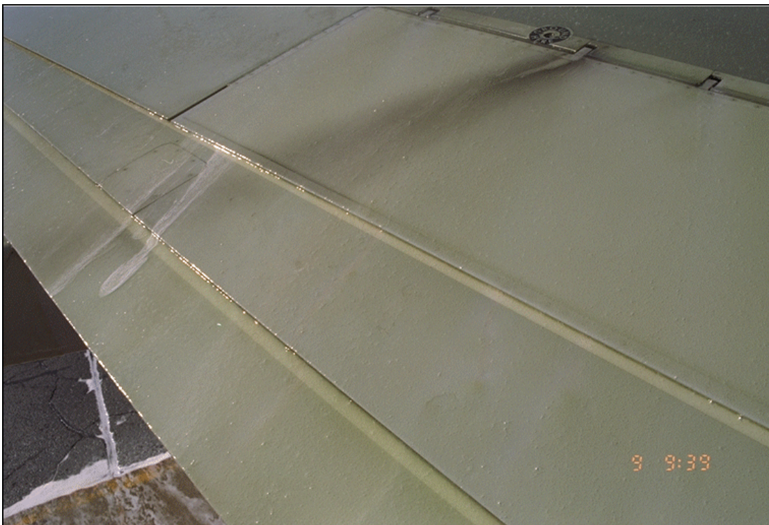
Photo 3.6: Akron Type I Nozzle – Type IV Fluid on Control Surfaces
