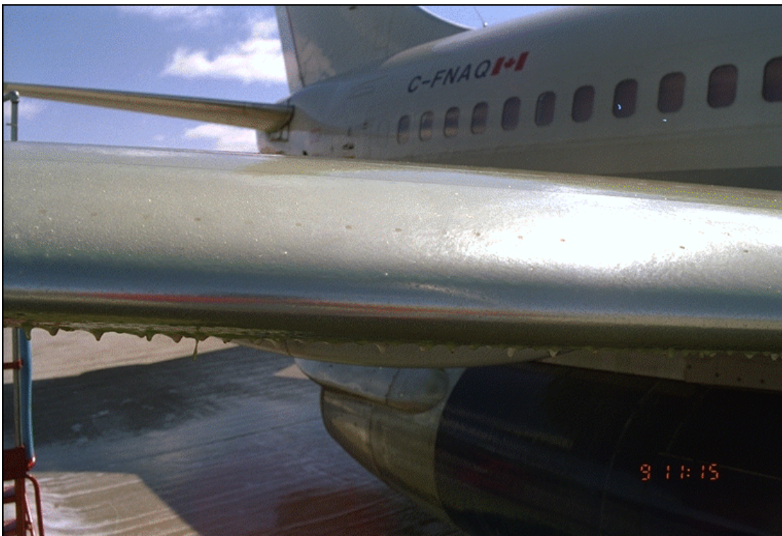
Photo 3.14: Elephant \beta – Ultimate Film Thickness Trial
