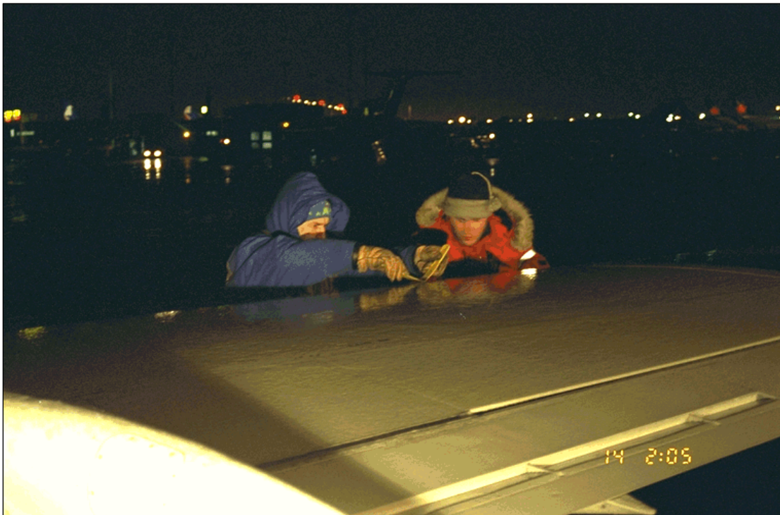
Photo 2.14: Collecting Samples of Fluid on Wing Surface
