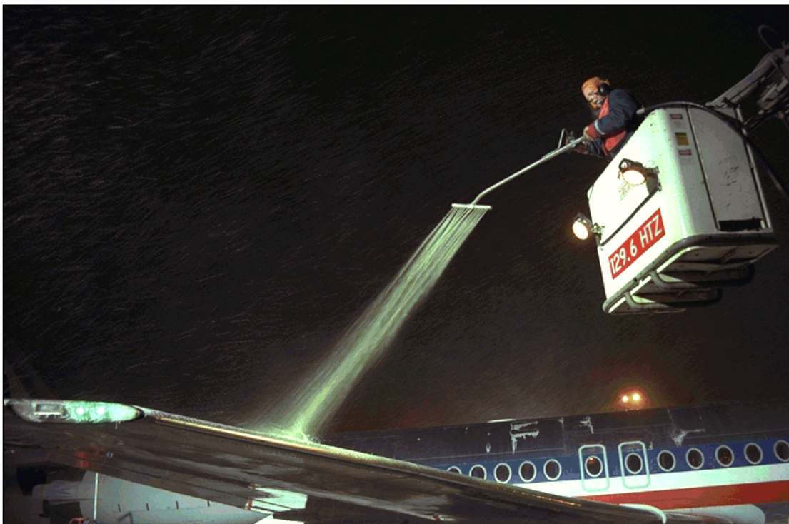
Photo 2.20: Spray Application with Wand
