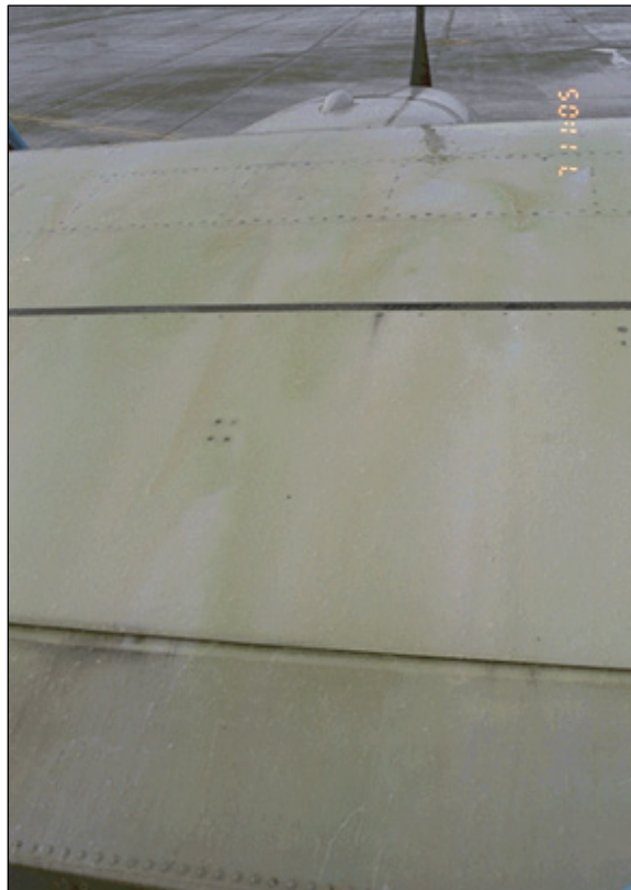
Photo 4.13: Appearance of Fluid in Propeller Wash Area
