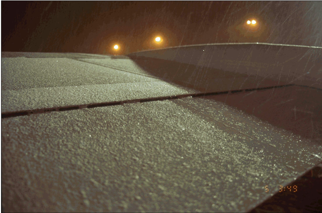
Photo 4.8: Fluid Failure Patterns on Fokker 100 Trailing Edge
