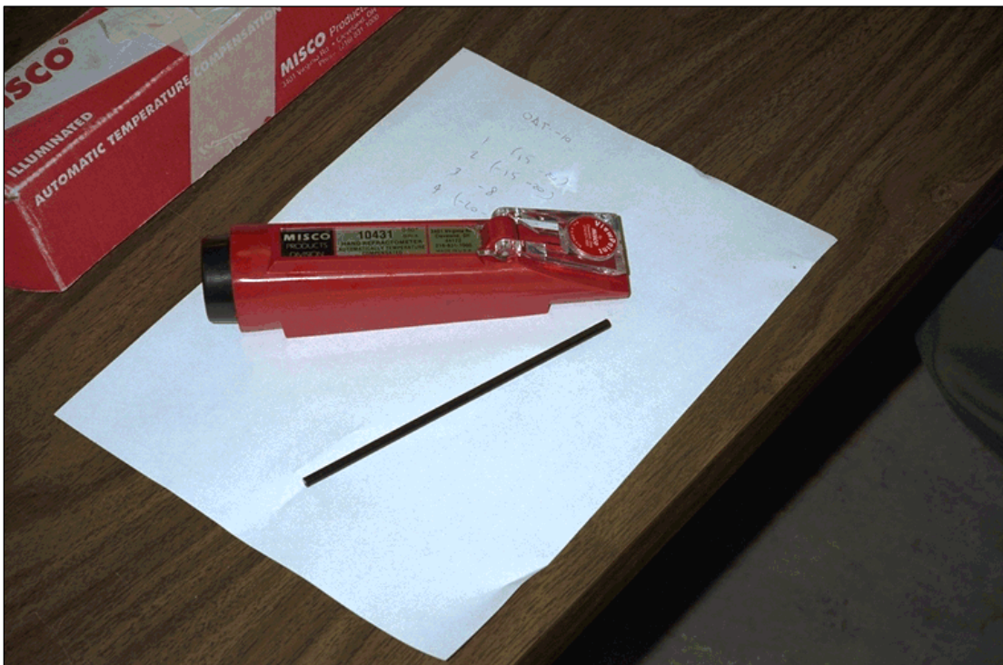
Photo 2.16: Misco Refractometer Used to Measure Freeze Point of Samples
