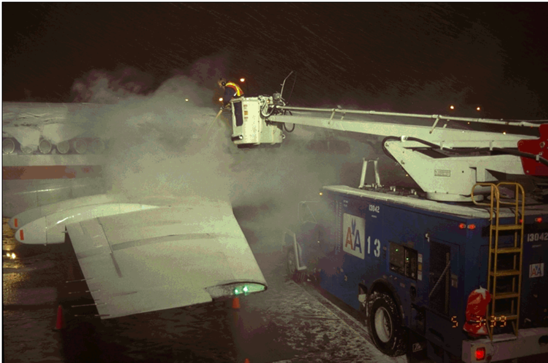
Photo 2.5: American Airlines Deicing Vehicle Applying Fluid on a Fokker 100
