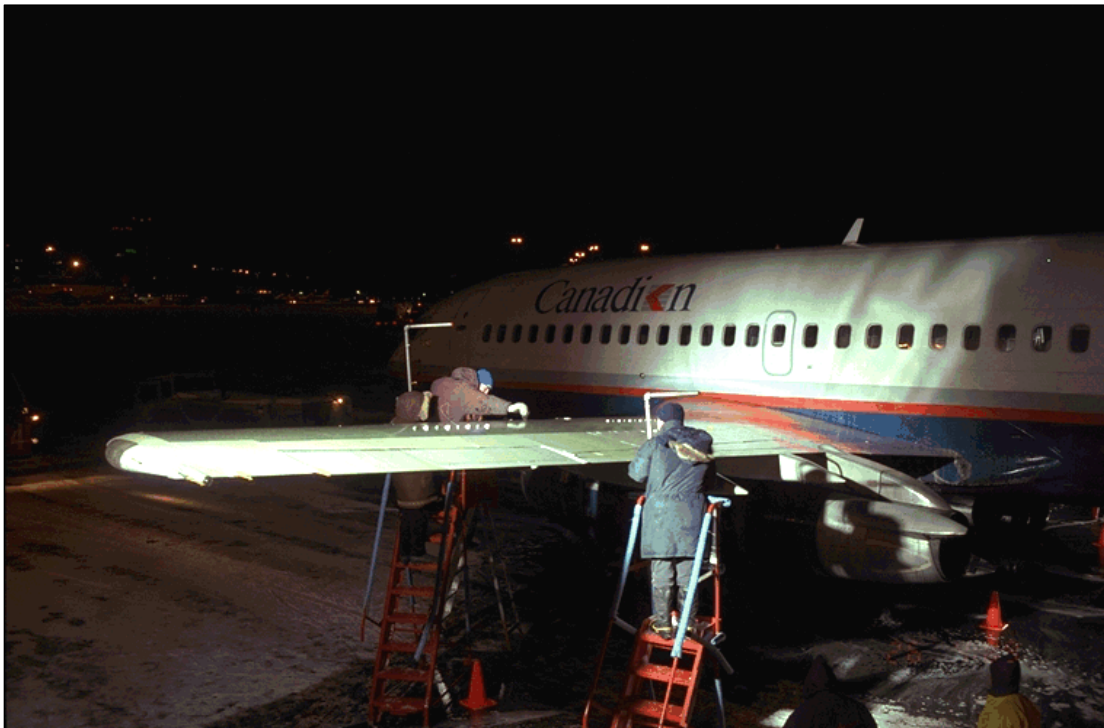
Photo 2.18: Measurement of Fluid Thickness
