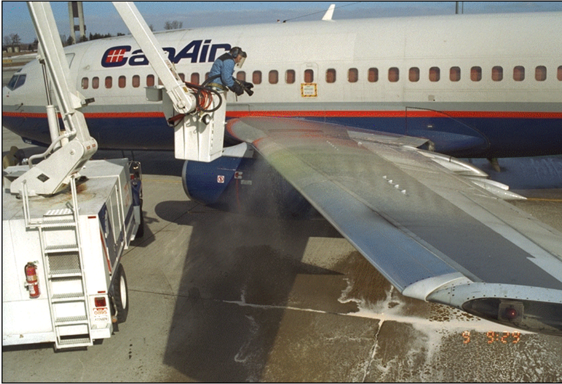
Photo 3.3: Akron Type I Nozzle – Type IV Fluid Application on Leading Edge
