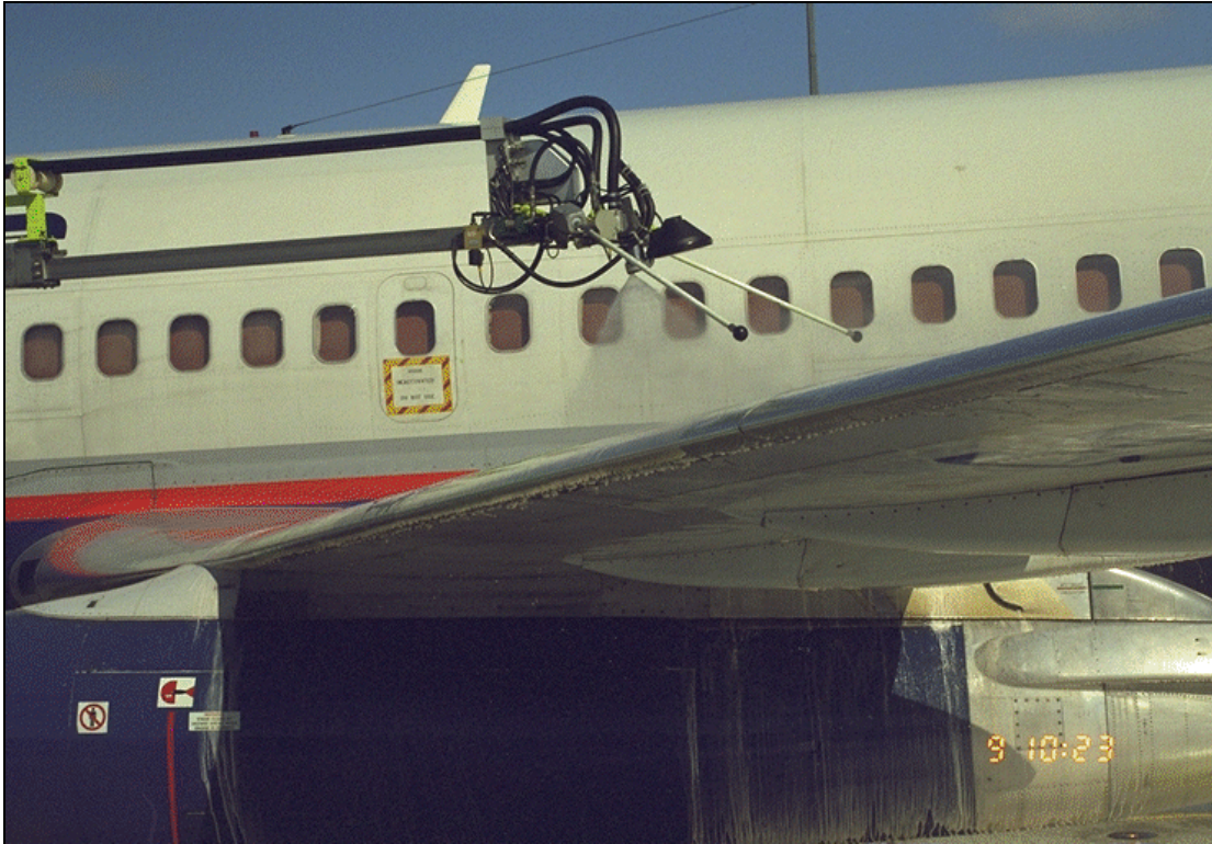
Photo 3.11: Elephant \beta – Optional Fixed Nozzle
