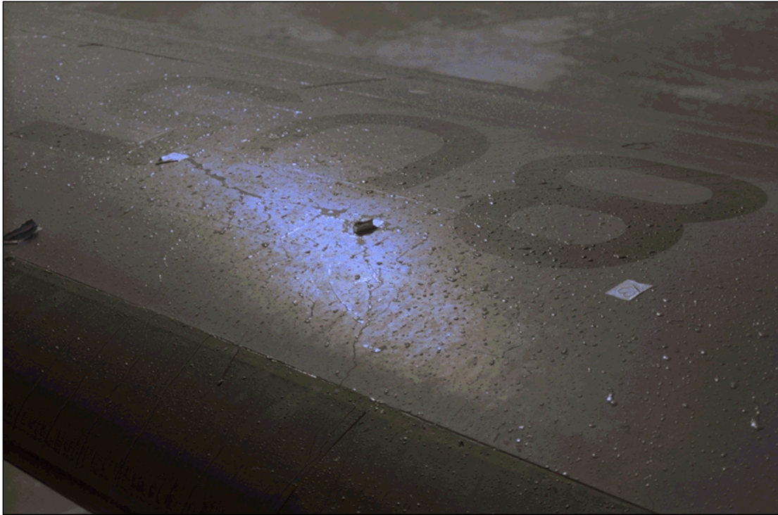
Photo 3.1: Fluid Beading on a DHC Dash 8 Wing
