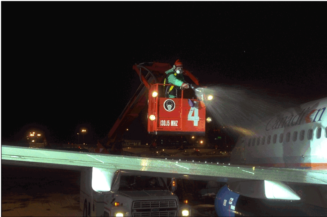
Photo 2.19: Spray Application with Task Force Tips Nozzle
