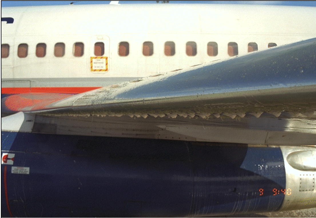
Photo 3.5: Akron Type I Nozzle – Type IV Fluid on Leading Edge
